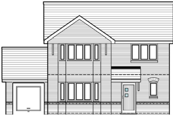
*Figure 3. Front Elevation – Harlech House Type*
